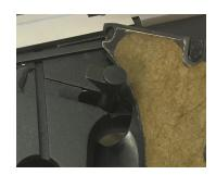
4. Start threading the included screw through the paddle button. Once it starts coming out the other end, screw it to the "Titan". Adjust button to your preferred position.
