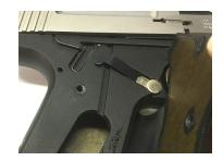
2. Remove the magazine release and release spring. The release spring is going to be reinstalled with the "Titan" Extended Mag Release.
